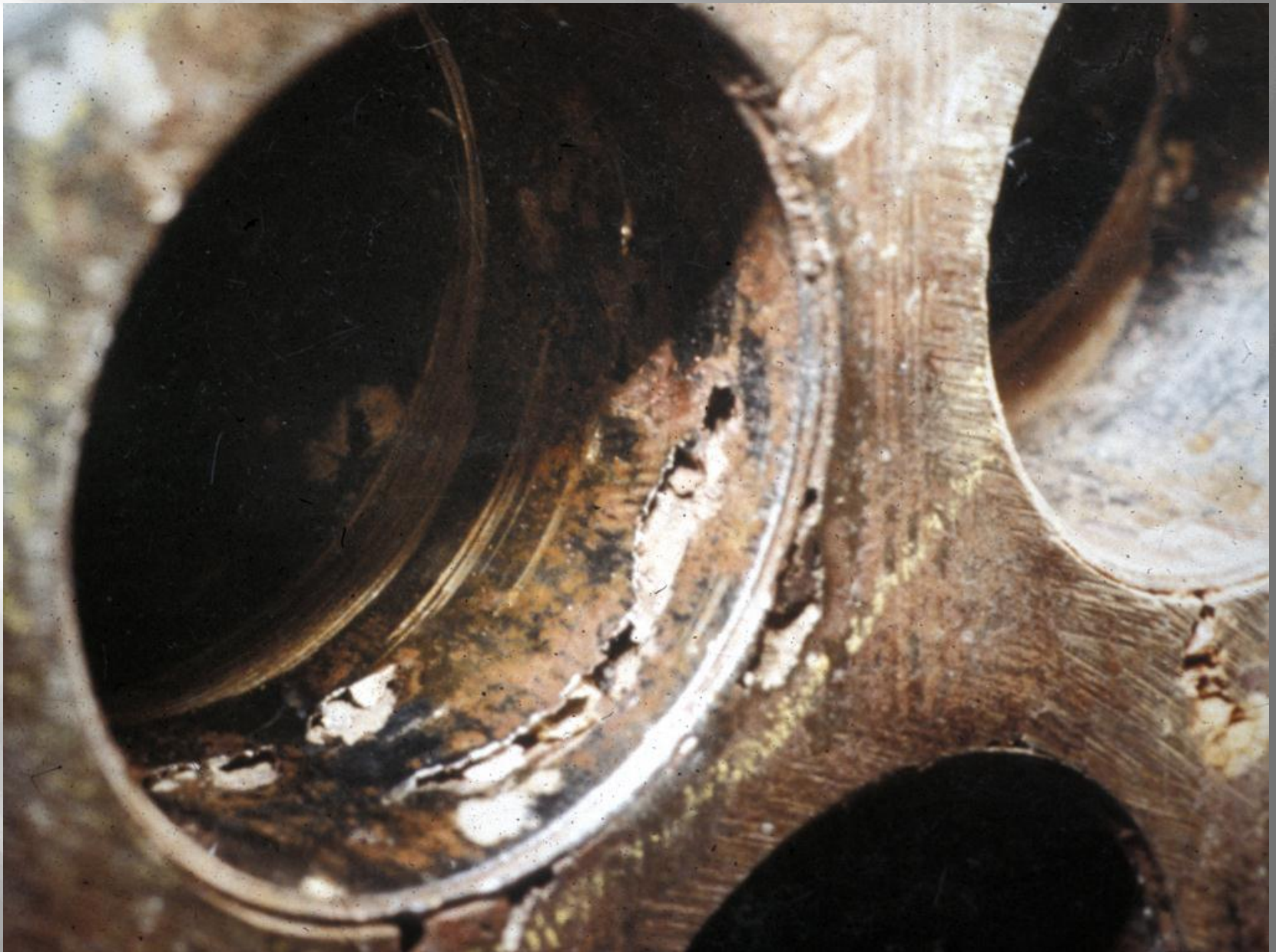
Crevice Corrosion and MIC on Stainless Steel
