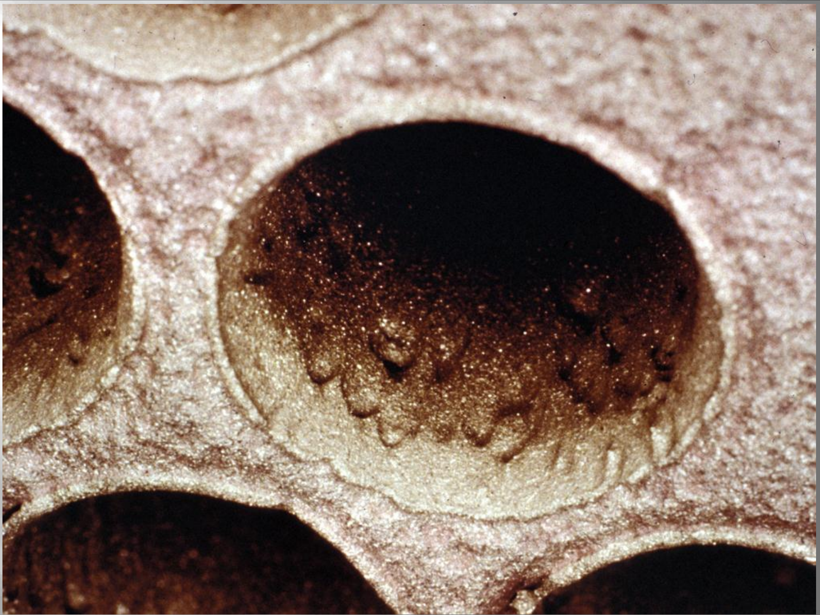
Inlet tube erosion on copper alloy tubes
