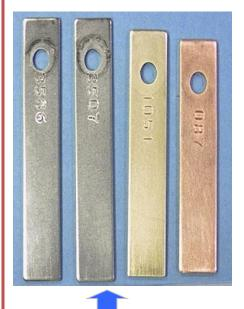
Test Coupons treated with GE Polyamine product
